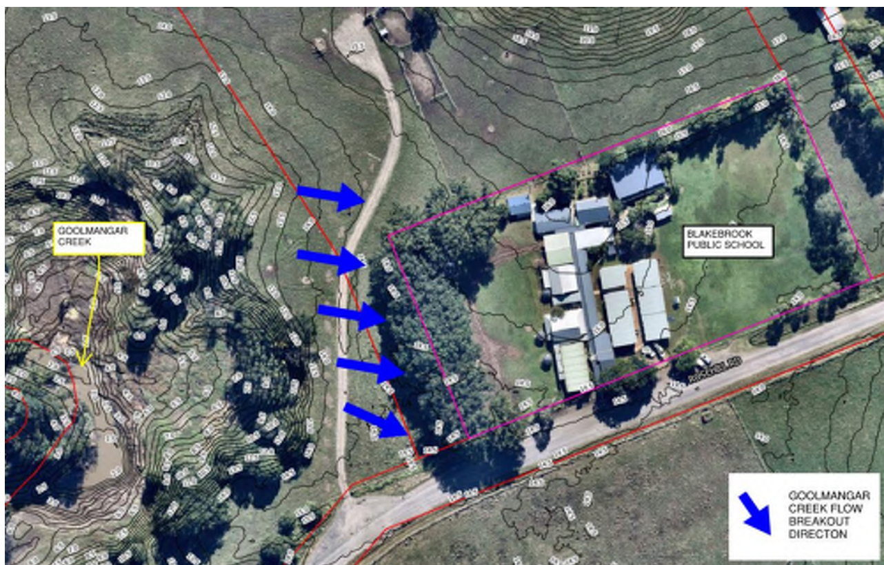
Figure 2-4 Indicative direction of flow of floodwater breakout from Goolmangar Creek
