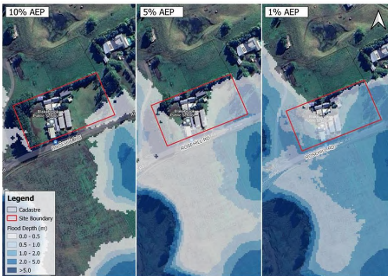
Figure 2-6 Flood depths in the vicinity of the school (Engeny, 2023)
